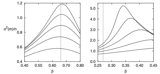
FIG. 3. Normalized fluctuations  $\sigma^2(m)/n$  versus inverse temperature  $\beta = 1/k_B T$  for ISAW on the square lattice (left) and the simple cubic lattice (right) at lengths 64, 128, 256, 512, and 1024. The curves for larger lengths are more highly peaked. The vertical lines denote the expected transition temperature at infinite length.
