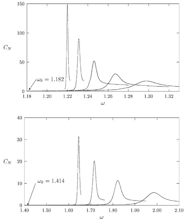
Fig. 2. Specific heat  $C_N$  versus  $\omega$  for interacting self-avoiding walks at lengths 1024, 2048, 4096, 8192 and 16,384 (above) and for interacting self-avoiding trails at lengths 512, 1024, 248, and 4096 (below) on the four-dimensional hyper-cubic lattice (Figs. 9 from [5] and 5 from [7]).
