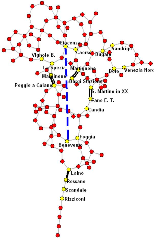
Fig. 3. The italian 380kV power grid with the most vulnerable edge (black thick line), the most vulnerable triple of edges (black double lines), and the edge that, if added to the network, improves the performance of the system best (dashed blue line). See tables. Nodes reported in tables are marked with a lighter color and with a label indicating the name of their respective substations.
