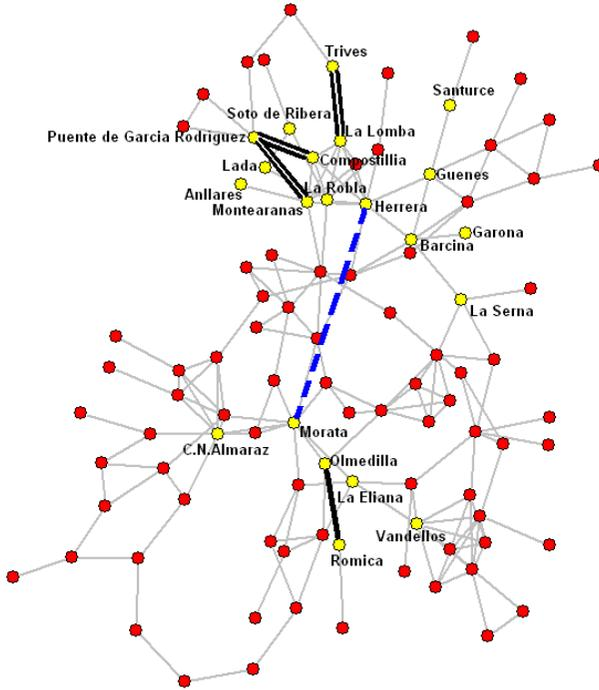
Fig. 1. The spanish 400kV power grid with the most vulnerable edge (black thick line), the most vulnerable triple of edges (black double lines), and the edge that, if added to the network, improves the performance of the system best (dashed blue line). Nodes reported in tables are marked with a lighter color and with a label indicating the name of their respective substations.
