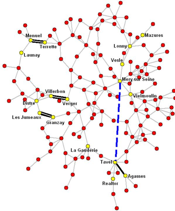
Fig. 2. The french 400kV power grid with the most vulnerable edge (black thick line), the most vulnerable triple of edges (black double lines), and the edge that, if added to the network, improves the performance of the system best (dashed blue line). Nodes reported in tables are marked with a lighter color and with a label indicating the name of their respective substations.
