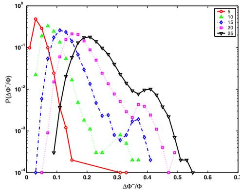
Fig. 5. Damage distribution in log-linear scale for the italian 380kV power grid, and for a number of removed edges equal to 5,10,15,20,25.
