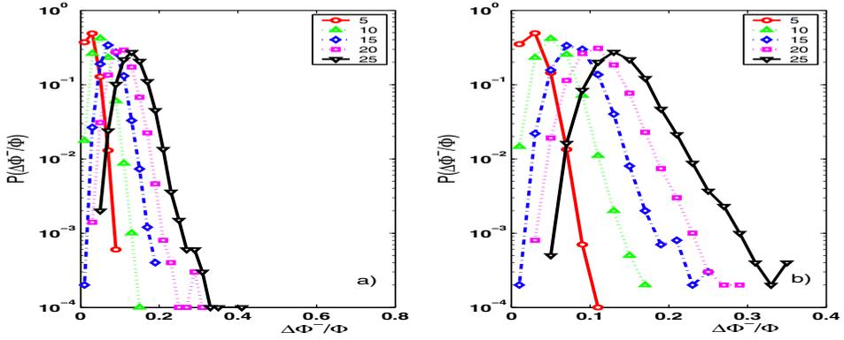
Fig. 4. Damage distribution in log-linear scale for a) the spanish and b) the french 400 kV power grid, and for a number of removed edges equal to 5,10,15,20,25.
