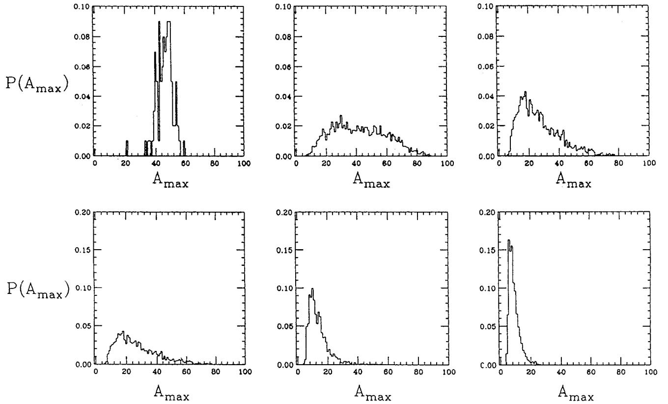
FIG. 5. We show the probability distribution of the size of the maximum fragment for six different initial temperatures for the  $A = 100$  fragmenting system in the CMD model. We observe that the width of the distribution attains its maximum at about  $T = 4$  MeV.
