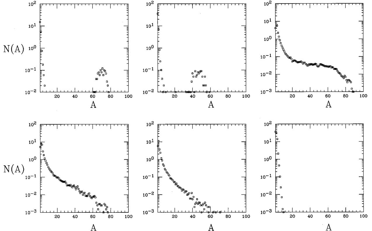
FIG. 1. Mass distributions obtained in the expansion of the system  $A = 100$  with six different initial energies, namely, 2, 3, 4, 5, 7, and 15 MeV g from 2 to 15 MeV (begining at the upper left corner).
