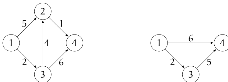
Figure 11.2: An iteration of Dijkstra's algorithm with t = 4 . In the graph on the left, c_{2t} = \min_{i \in V \setminus \{t\}} c_{it} and therefore, by Lemma 11.1, \lambda_2 = c_{2t} = 1 . The graph on the right is then obtained by removing vertex 2 and updating c_{14} to \min\{c_{14}, c_{12} + c_{24}\} = \min\{\infty, 5 + 1\} = 6 and c_{34} to \min\{c_{34}, c_{32} + c_{24}\} = \min\{6, 4 + 1\} = 5 .
