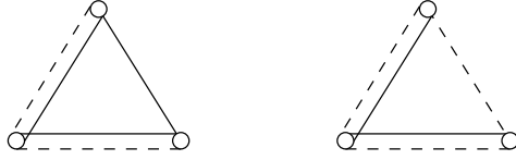
Figure 4: The two mixed circuits on three vertices. These graphs, denoted by K_3^+ and K_3^- , are the smallest (mixed) circuits of the direction-length rigidity matroid.
