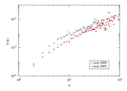
Fig. 3. Average betweenness b(k) of nodes with k links, as a function of k for the years 2000 and 2005. The straight lines are power-law fits  $b(k) \sim k^{\eta}$  with an exponent  $\eta$ , respectively, equal to 1.4 (dashed line) and 1.6 (dotted line).
