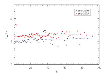
Fig. 4. Average degree  $k_{nn}(k)$  of nearest neighbors of nodes with degree k, as a function of k. Results refer to year 2000 and year 2005. The two dashed lines are fitting to the data, with slopes v respectively equal to 0.005 and 0.006
