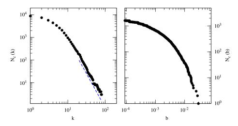
Fig. 2. Left panel. Cumulative degree distribution (year 2000): the number of nodes  $N_c(k)$  with degree larger or equal to k is reported as a function of k. The line is a power law  $N_c(k) \sim k^{-(\gamma-1)}$  with an exponent  $\gamma - 1 = 3$ . Right panel. Cumulative node betweenness distribution (year 2000): the number of nodes  $N_c(b)$  with betweenness larger or equal to b is reported as a function of b.
