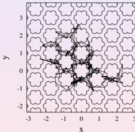
similar settings for electrons in semiconductor **antidot lattices** and for diffusion in **porous media**
